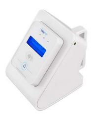
The device can be placed onto a table top and used as a 'static' donation point. If so, it will need to be secured to the wall or a piece of furniture using a security cable (advice can be provided on this, please ask).
